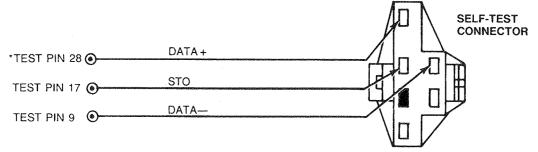
\*TEST PINS LOCATED ON BREAKOUT BOX HARNESS CONNECTOR VIEWED INTO MATING SURFACE.
