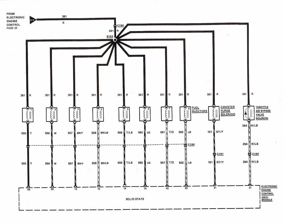
The 5.0L SEFI engine uses EEC IV Sequential Fuel Injection (SEFI). Fuel is injected directly into each cylinder through the Fuel Injectors in a sequential manner. Fuel is supplied up by an Electric Fuel Pump. With the Ignition Switch in START or RUN, the EEC Power Relay applies voltage to the circuit. When controlled by the EEC Module, and with the Inertia Switch closed, the Fuel Pump Relay operates, applying power to the Fuel Pump.
